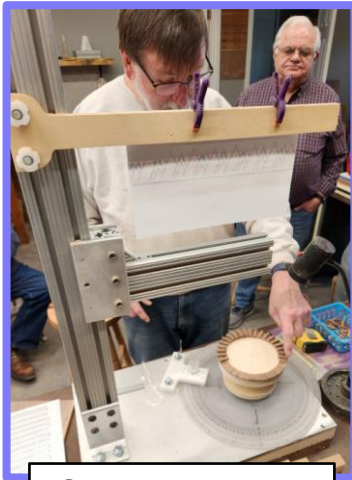
Gluing with the jig
