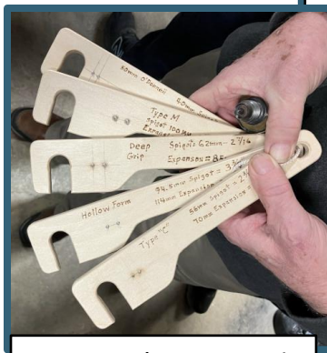
Dan Ernst's tenon and recess marking gauges
