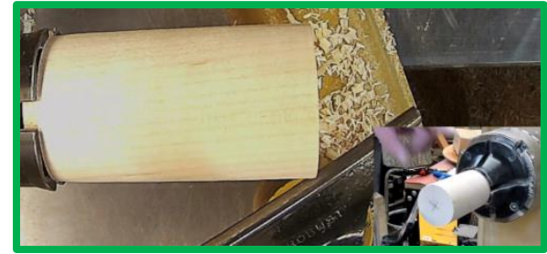
Dick Hicks mounts the blank in the chuck to do the top ; 30° degree angle for the top
