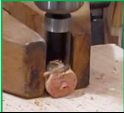
Cutting cork with a plug cutter
