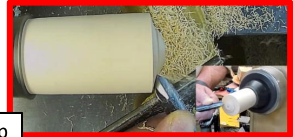
Dick Hicks mounts the blank in the chuck to do the top ; 30° degree angle for the top
