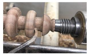
With the ring tool, undercut each of the three rings. Alternate from one side to the other until ring is free.
