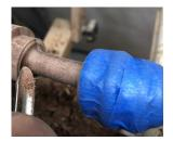
With a caliper set to 1/2", turn the shaft to its final finish. Use a spindle gauge to create a cove in the corners of each end of the shaft. Taping the rings in place can keep the rings out of the way.
