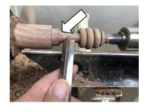
With a gauge, level off the shaft. We'll turn it to its final diameter later, Move the rings to level the full length of the shaft.
