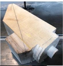
hole bored for a 1 ¼" number 10 set screw through chuck into the bottom. That will come into play in step 4. This will fit on the Escoulen chuck made by Vicmark.
